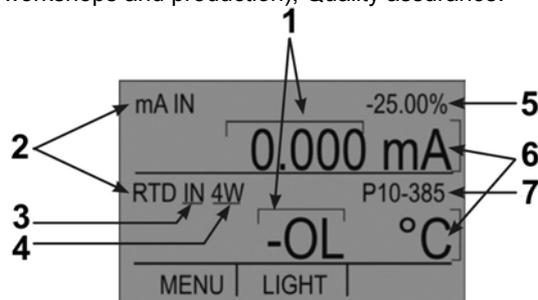
The handling of the **LEC 200** is very easy. Arrow keys, direct numeric keypad entry, and three software-driven function buttons, plus a large backlit, menu-driven graphics display combine to provide a highly intuitive, simple yet powerful operator interface.
