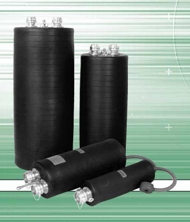
**Pipe stoppers** are made of quality rubber reinforced with nylon or kevlar fabric. The metal parts are made of stainless materials. Each pipe stopper is provided with quick coupling for inflation and eyebolt for removing and blocking. They withstand weather, temperature from -30 °C to 80 °C, use and waste water and they are middle resistant of chemicals. They are mainly used during repair and maintenance works, accidents and for the leak tests with water or air.
