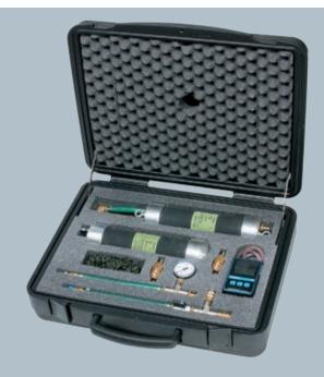
This set is used for DN 80 to 150 mm pipe leak tests using air as the testing medium. They can be used both in straight sections of the pipe and in section with round or sharp bends or knee pieces up to 90 degrees. The set consists of a digital pressure gauge and all the necessary fittings and accessories for carrying out leak tests according to DIN EN 1610.
