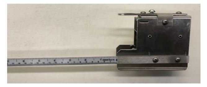
3. Insert the spacer bar into the left bracket, and position the bracket at the separation distance referenced earlier. Tighten the spacer bar clamp at this position:
