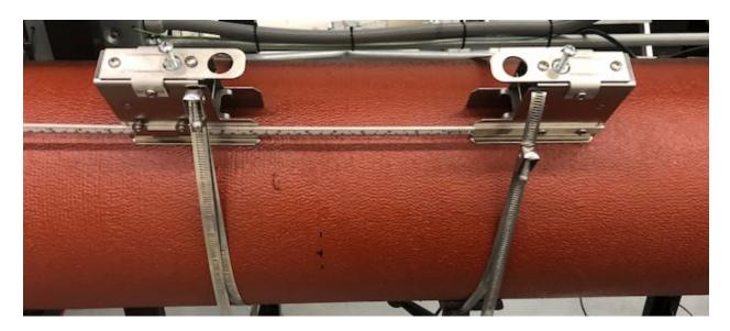
5. Apply coupling compound to the transducers, and install them in the brackets.
