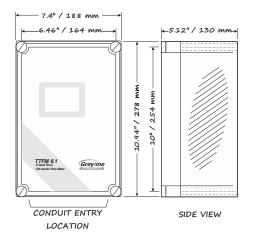
Note: This non-metallic enclosure does not automatically provide grounding between conduit connections. Grounding must be provided as part of the installation. Ground in accordance with the requirements of the National Electrical Code. System grounding is provided by connecting grounding wires from all conduit entries to the steel mounting plate or another point which provides continuity.
