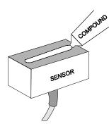
Use the pipe clamp and rail (supplied) as illustrated on previous page. Apply Super Lube® to the colored face of the sensor. A bead, similar to toothpaste on a toothbrush, is ideal. Do not overtighten (crush the sensor).
