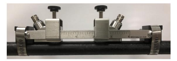
5. If you need to make fine adjustments  $(\pm 0.1^{"})$  to the spacing at this point, you may do so by loosening the tightening screw slightly, sliding the second transducer, then re-tightening it.
