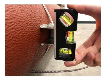
5. Mark the position of the center line of the bracket which is to be moved to the opposite side of the pipe. It is up to you to determine which bracket is easier to move from the current position:
