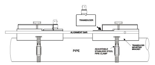
Mount the Mounting Bracket as illustrated on pipes 2" / 50 mm OD or larger. Stainless steel bands are included for mounting on pipes up to 30" / 750 mm OD.
