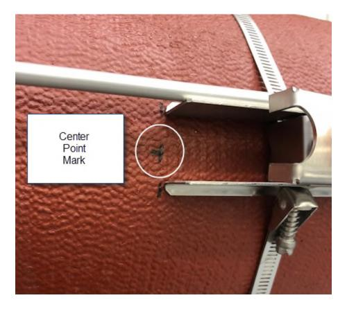
5. Measure the separation distance from the marks you created in step 4, and create new marks on the pipe at the separation distance. It may be useful to mark your Greyline tape measure at the separation distance before holding it up to and marking the pipe.
