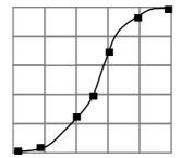
You should enter 2 level/volume breakpoints at the minimum and maximum levels, and several for each place where the vessel has got an arc. You can enter any number of pairs between 2 and 16.
