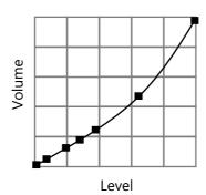
You should enter a level/volume breakpoint for each place where the vessel changes direction, and numerous where the section is slightly curved (mostly linear but has got a small arc). You can enter any number of pairs between 2 and 16.
