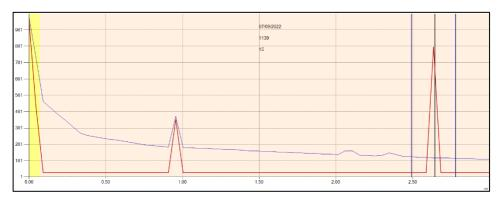
To zoom out, simply draw a box from the bottom right to top left and the echo trace will resume its normal shape.
