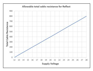
Maximum cable resistance vs supply voltage.
