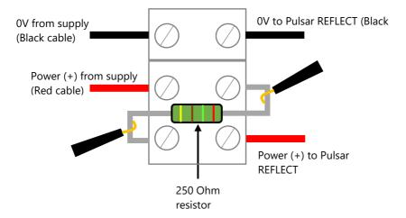
To enable the Pulsar REFLECT Intelligent Transducer to work correctly, the power (red) cables from the supply and to the REFLECT must be wired in series with the 250 Ohm resistor (as seen in the above picture).
