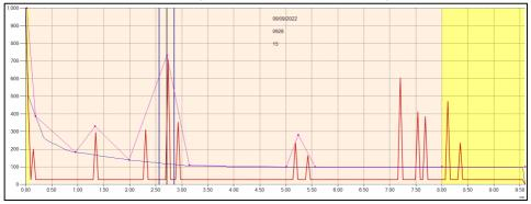
The points can be clicked on and dragged in order to manipulate the DATEM line to cover any unwanted echoes you want to hide from the echo selection algorithm. Once the line is in its final position, click the
